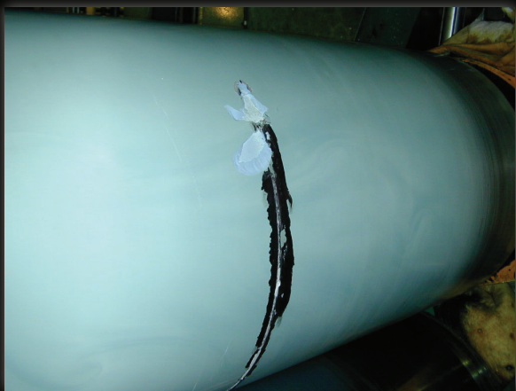
Typical damage caused by an undetected hot spot
