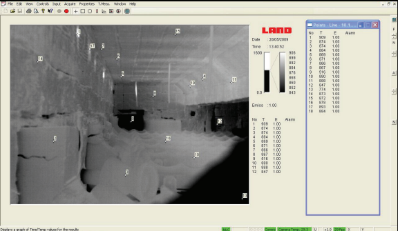
Point temperature measurement inside the furnace
