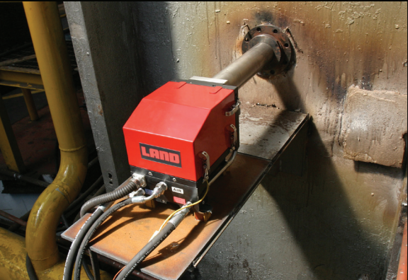
Typical installation showing the FTI-Eb mounted into a process - the sensor is shown in the protective enclosure
