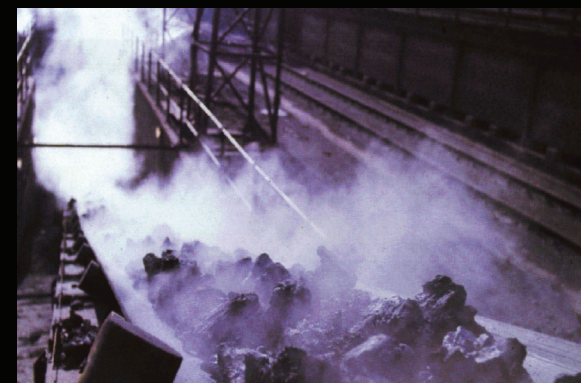
Hot Coke Conveyor
