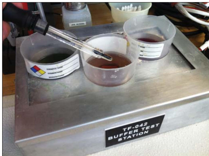
Great example of a two point calibration station. Two buffers and rinse water. An example of a laboratory style pH electrode can also be seen in this photo.
