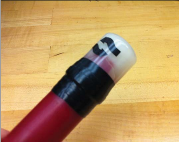
A pH sensor with liquid filled cap prior to shipment. The black electrical tape helps to secure the cap and prevents leakage.
