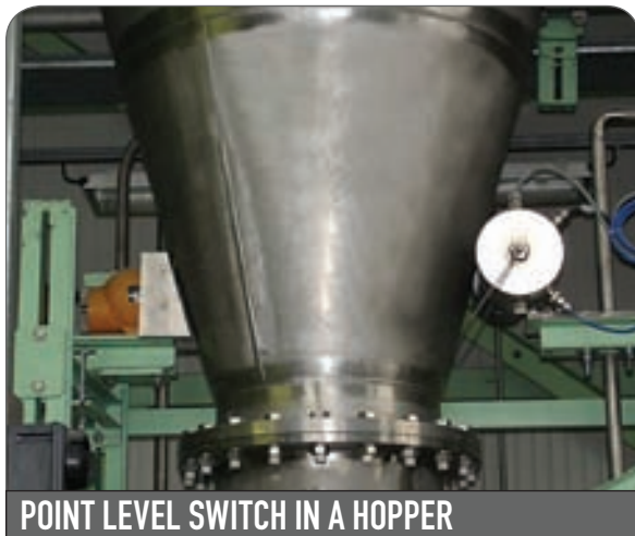
Figure 4. A narrowly collimated conical beam is aimed across the vessel at the point detector.
