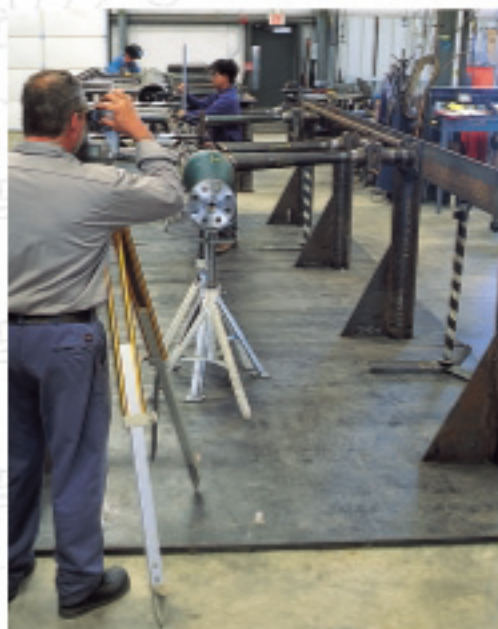
(Above) CSI Production Crew Leader uses a transit to maintain close tolerances (.010") in the production of polymer manifolds.
