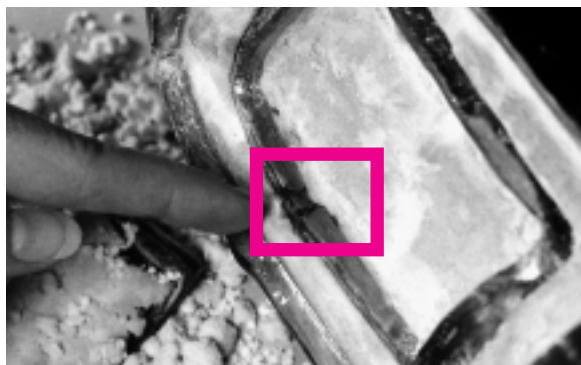
Heat affected zones adjacent to welds are "weak links" in jacketed piping systems. That's where stress fractures occur most frequently. The result is cross contamination, shown above in a sulfur transfer line. Sulfur breached the jacket annulus.
