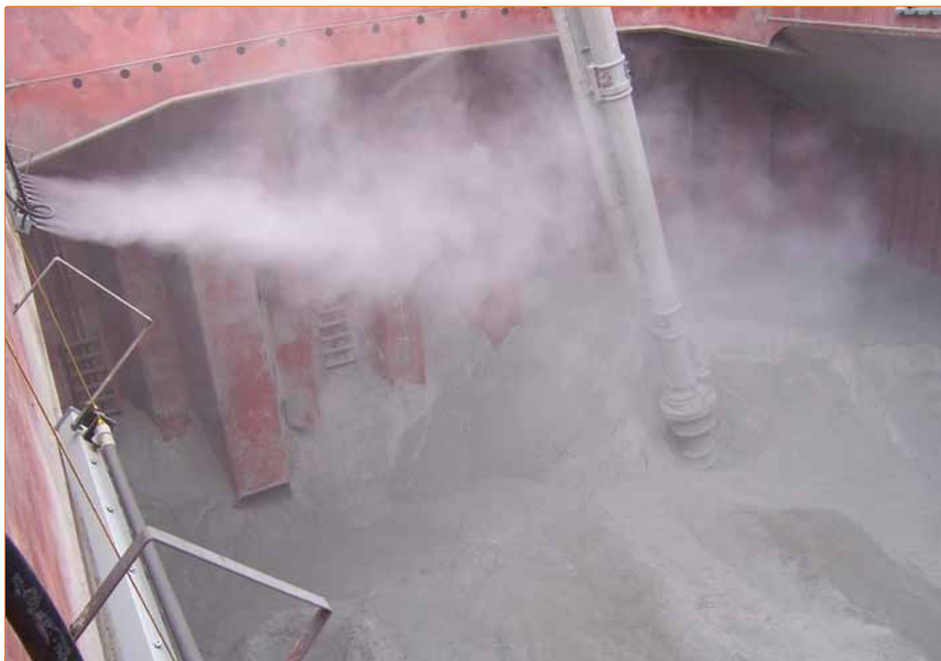
Figure 4. Fogging systems such as the Dry Fog system has been designated a Best Demonstrated Technology by the U.S. Environmental Protection Agency (EPA).
