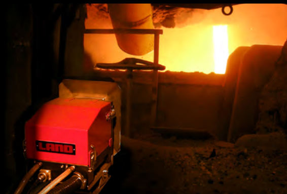
The Slag Detection System has a robust housing assembly, which views directly the liquid metal stream as the steel is tapped.
